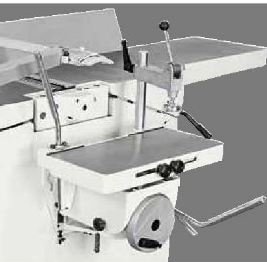
Cast-iron mortiser Drilling holes and mortises are easily carried out. It includes the exhaust hood, 120 mm diameter and 16 mm chuck.
