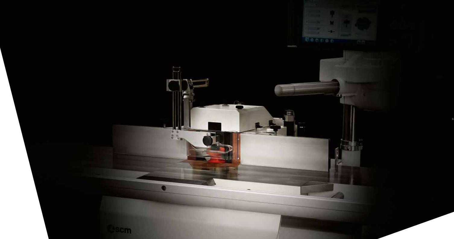
Speed of setting-up due to the unique movement mechanism of the spindle (SCM patent), which enables the operator to position independently the height of the tool with the tilted spindle and the moulder fence. Maximum performance using the latest technology of the screws with recirculating ball-bearings and the linear guides which guarantee a total absence of vibration and wear, therefore much reduced maintenance (centralised lubrication).
